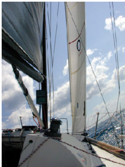
Code 2 Jib in 9 knots true wind, with clew pulled 50-75mm inboard.
