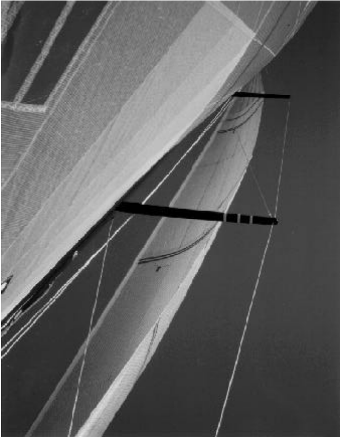
Median Twist Profile: CODE 2 jib max trim bottom, 375mm inside lower spreader, with top twisted slightly 325mm inside top spreader. 15 knots true wind, lead aft 25mm from median.
