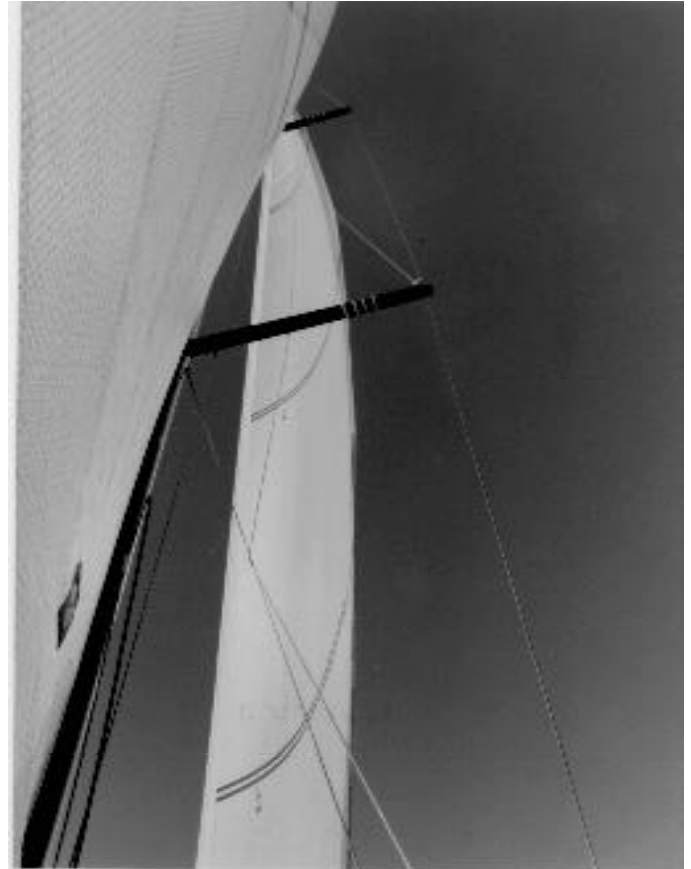
Tight Twist Profile: CODE 2 jib 12 knots true wind trim 375mm (15") at top and bottom spreader, lead at median.
